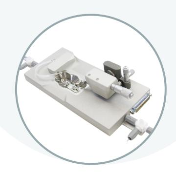
The Pressure or Perfusion Myograph System - 114P is a system used to study the structure and function of isolated sections of small vessels (diameter >40  $\mu$ m) under near physiological conditions. Vessel diameters can be measured in response to pharmacological and physiological stimuli.
