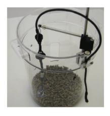
Conscious Animal Enclosures provide a convenient environment for using the MouseOx® Plus to monitor or collect data on conscious mice or rats.
