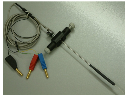
SEN-12 360° ball manipulator with stimulating electrode
