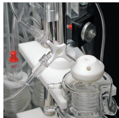
Additional ports on the Junction Block allow easy introduction of experimental drugs.
