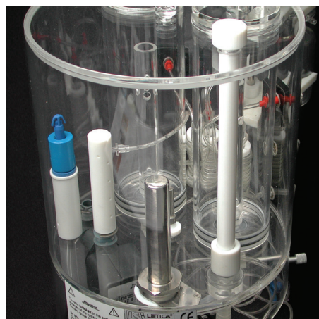
Sensitive temperature and water level sensors provide accurate temperature maintenance.
