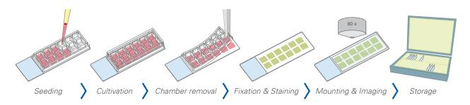
In the ibidi <u>Chamber Slides</u>, a silicone gasket with separated chambers is mounted on a standard glass slide. The ibidi Chamber Slides for immunofluorescence are ideal for the long-term storage of samples that are mounted with a glass coverslip.
