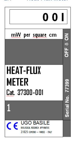
The Meter upper panel features a 3-digit display which indicates the heat-flux, whose measuring unit (mW per square cm) is indicated below the display window.
