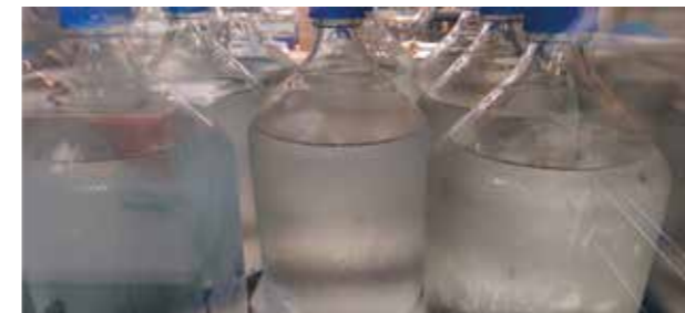
Condensation on the bottles during transport from the cool room to the air lock
