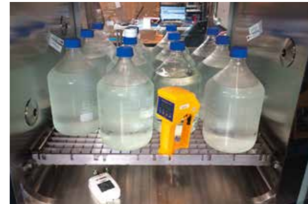
Drying phase of the condensate before H 2 O 2 decontamination
