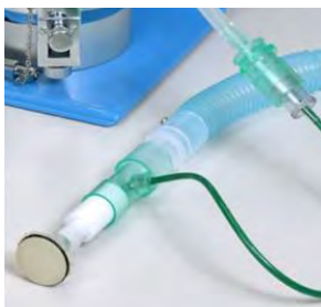
The picture shows a mouse nose-cone/mask, connected to an evacuation tubing.
